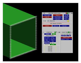
Create a set of nodes called fixed\_end\_of\_box – as shown above and restrain all degrees of freedom as shown below.
