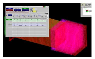
We now define an initial velocity for the set "initial\_velocity" of 20e3mm/s.
