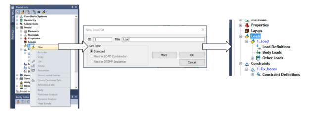
With that complete we then define the actual load. Select the on surface option. We then select the geometry that we are going to apply the load to. In this case it will be the surfaces on the internal faces of the end bore.
